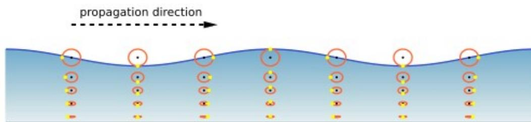
*Illustration 3: A wave through water, showing anticlockwise movement of particles, (Kraaiennest, 2008)*
