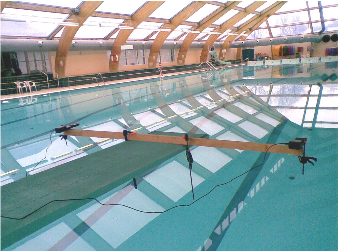
*Illustration 7: The apparatus, showing the two sensors at opposite ends of the plank, pointing down towards the water surface one metre below.*
