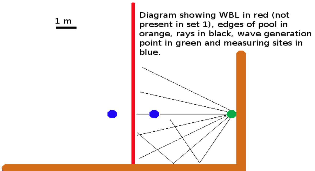
*Illustration 8: Diagram (approximate scale) showing significant features of experiment #3 at water level.*
