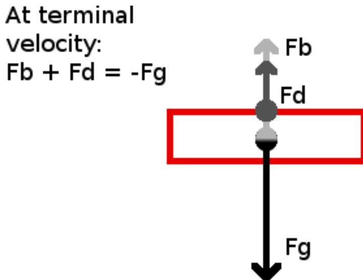
Illustration 5: Diagram showing forces acting on disc as it sinks through water, with points of application.
