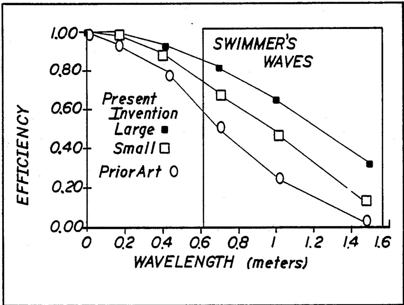
Illustration 9: "Efficiency" of WBLs at different wavelengths. (Kiefer, 1990)
