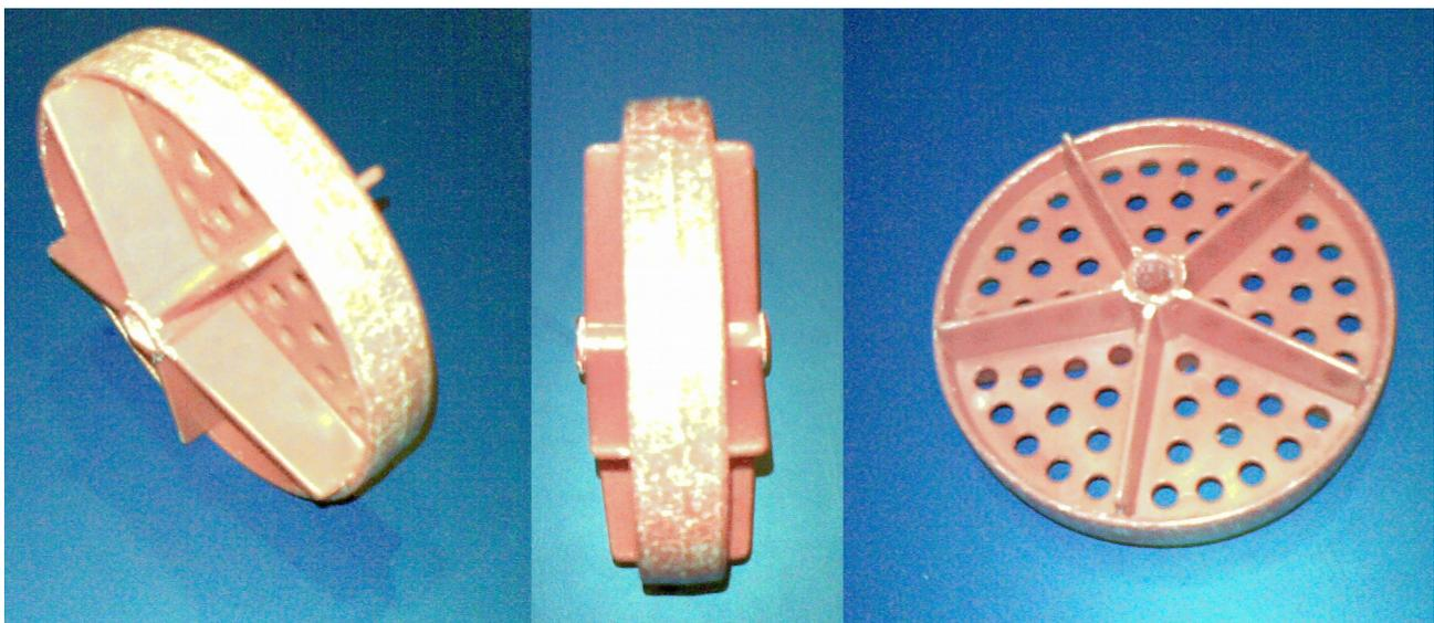
*Illustration 2: A single disc from the type of wave breaking laneline studied, from three angles. For physical data about the disc, please see Appendix 2: Data about a single disc.*
